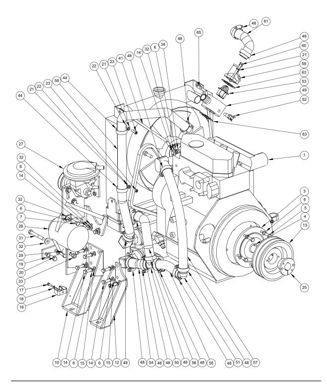
Figure 1-41 **Daihatsu Engine Assembly - Maxx 450 Diesel - View 2** D-6056 Rev A
