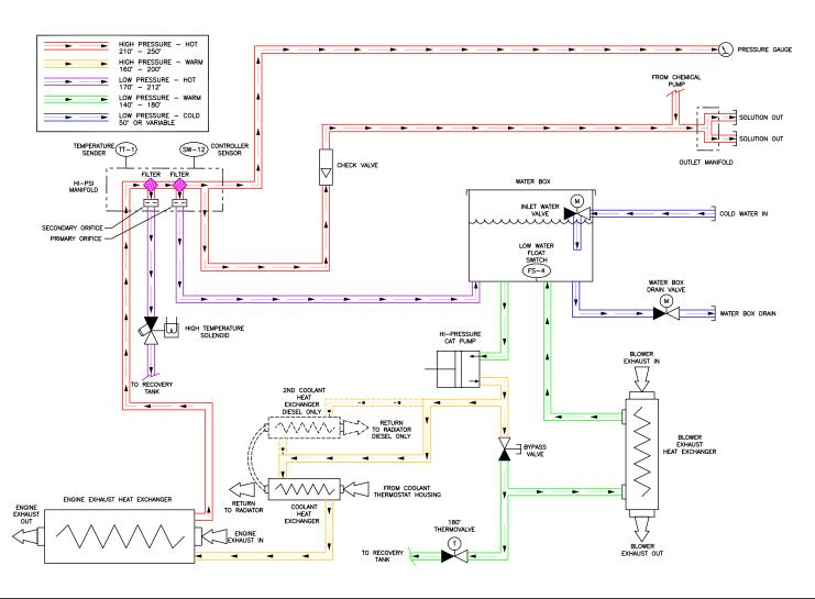
Figure 5-2 **Chemical System Flow Diagram** D4382 Sht 2 Rev A
