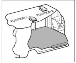
Figure 1-1 Roof Vent
