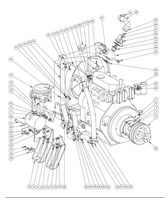
Figure 1-32 Maxx 450D Daihatsu Engine Assembly - View 2 D-4351 Rev G
