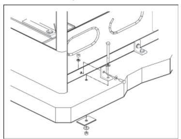
Figure 1-3 Installation Using Tie-down Cleats
