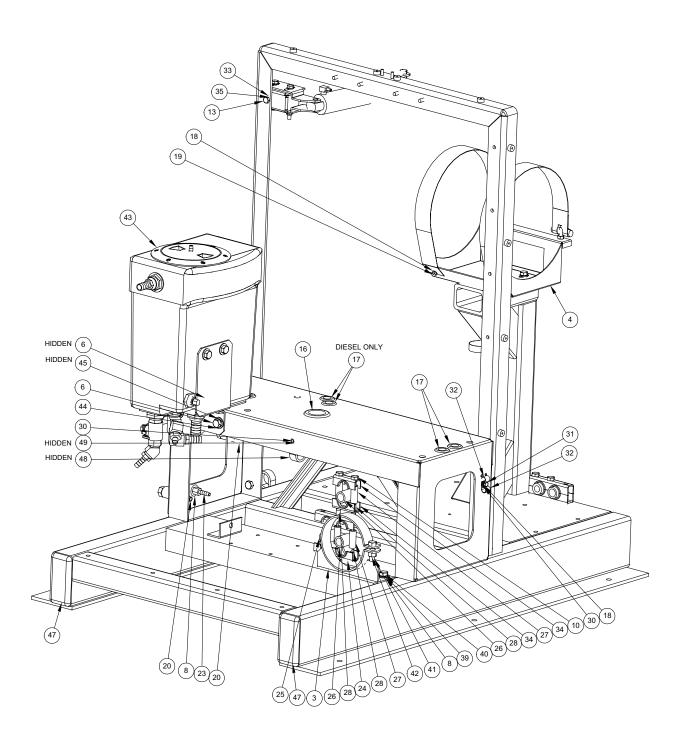
Figure 1-8 Maxx 450D/470D Frame Assembly - View 2 D-4355 Rev F
