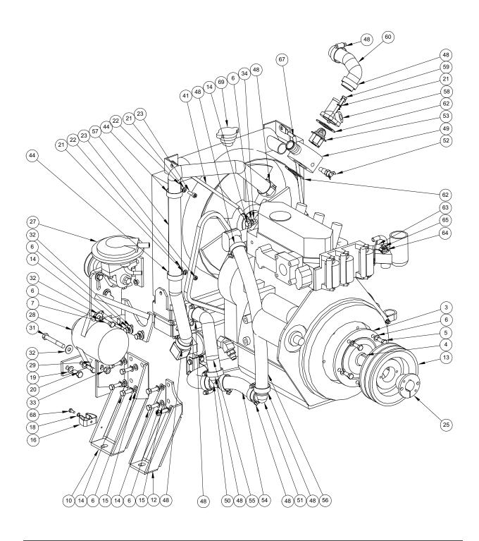
Figure 1-34 Maxx 470D Daihatsu Engine Assembly - View 2
