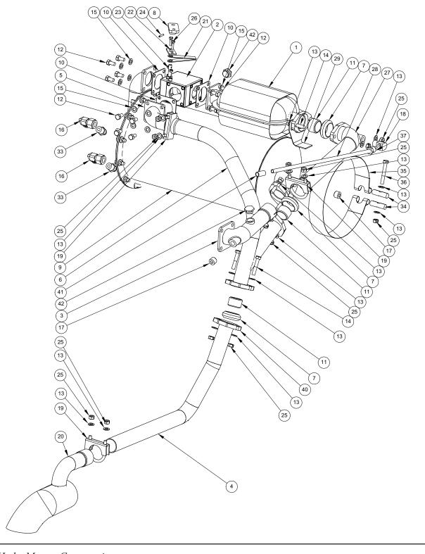
Figure 1-28 **Exhaust Assembly - View 2** D-4541 Rev F
