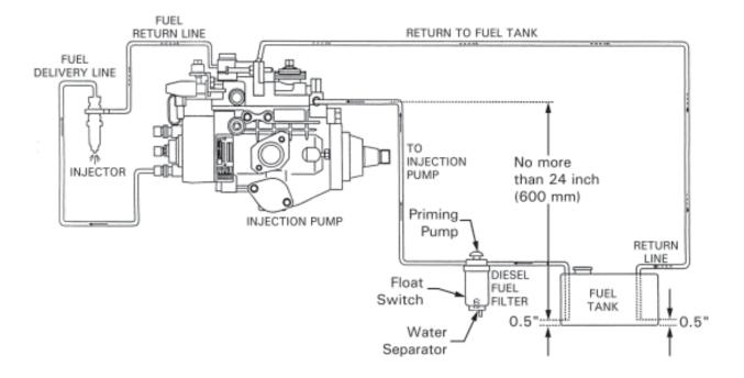
Figure 4-2 Diesel Fuel Filter with Manual Priming Pump, Water Separator with Electric Motor
