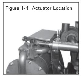
If the poppet **seats** in both directions, the the diverter actuator is in proper adjustment.
